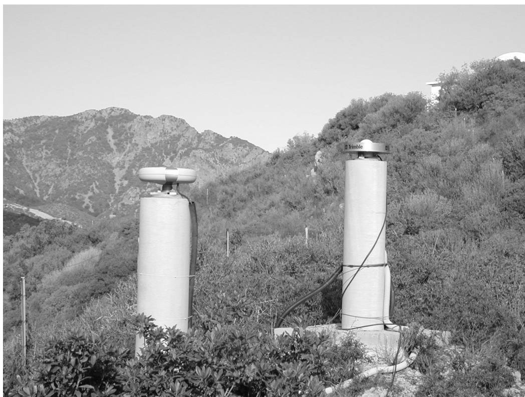
Figure 6 – To the left the RMB2 pillar with the RegAnt 2 antenna, to the right the ASI reference station
