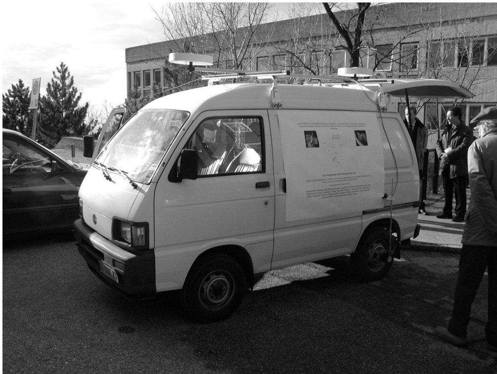
Figure 5 - GIGI (Gps Integrated with Glonass and Inertial navigation system)
