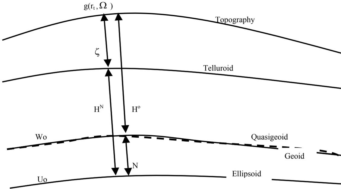
Figure-1: The geoid undulation( $N$ ), Orthometric heights ( $H$ ), Height Anomaly ( $\zeta$ ) and Normal heights ( $H^N$ )
