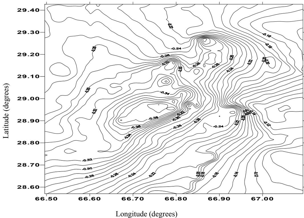
Fig-7. Geoid to Quasigeoid separation term C2 from observed gravity data in Kalat Area. Contour Interval=10 mm
