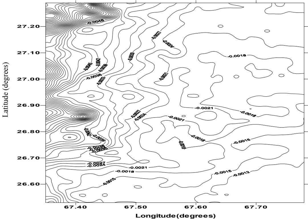
Fig-6. Geoid to Quasigeoid separation term C2 from observed gravity data in Dadu Area. Contour Interval=0.3mm
