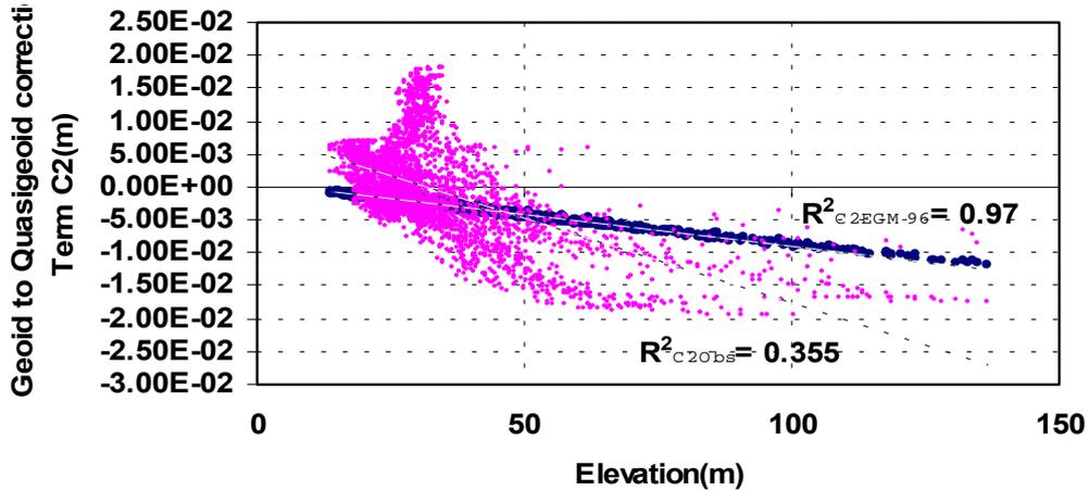
Fig-5. Relationship of Elevation with geoid-quasigeoid correction C2 term from observed gravity data and EGM96 model gravity in the Dadu area
