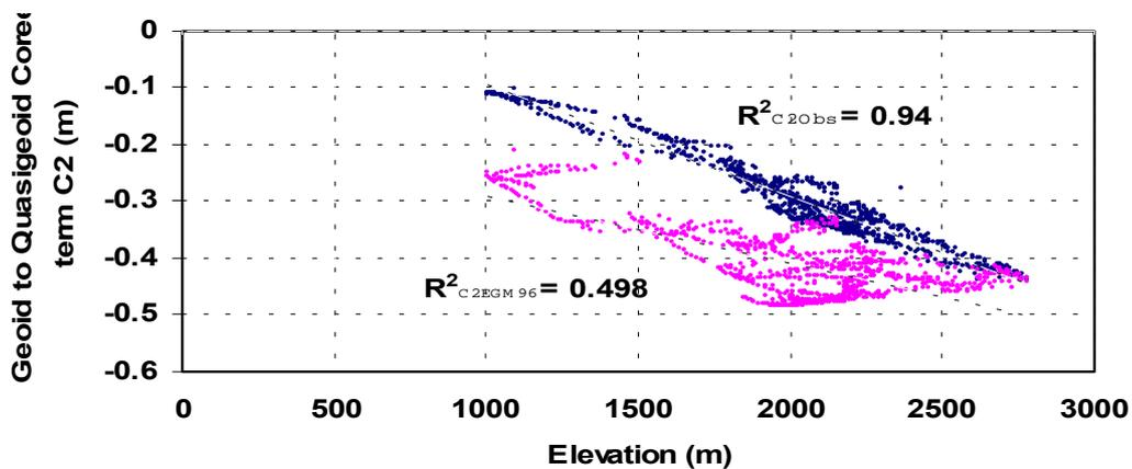
Fig-4. Relationship of Elevation with geoid-quasigeoid correction C2 term from observed gravity data and EGM96 model gravity in the Kalat area
