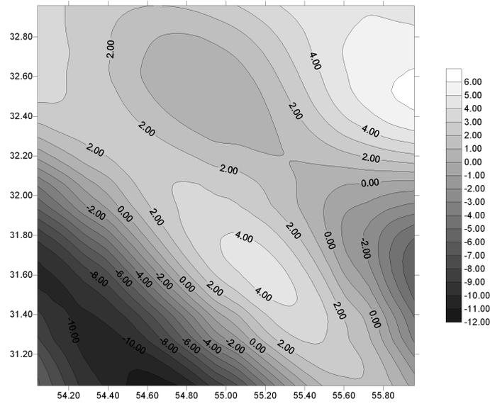
Figure 8: The primary indirect topographic correction computed by the spherical harmonic approach of Nahavandchi and Sjoberg (1998). Contour interval = 1 cm
